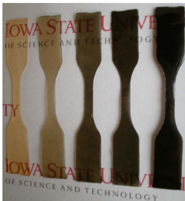
Figure 7. PU and PU/s-MWCNT nanocomposites (from left to right: with 0%, 0.2 wt %, 0.4 wt %, 0.8 wt %, 1.2 wt % s-MWCNT). [Color figure can be viewed in the online issue, which is available at wileyonlinelibrary.com .]
